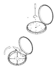
Step 4: Put cable through the entrance hole and connect it to the terminal block. Adjust the CCT as per the requirement 3000k/4000k/5700k
