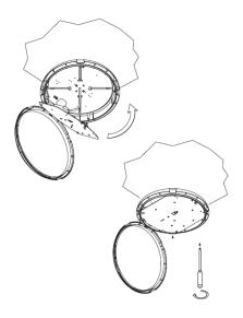
Step 7: Close the diffuser and lock the clips.
