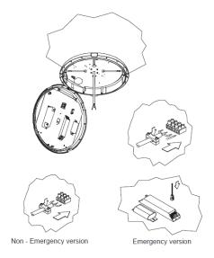
Step 5: Position and fix the base onto the ceiling
