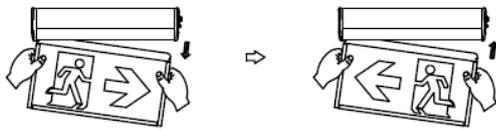
2. If need replace pictogram on EXIT sign panel, take off EXIT sign panel, disassemble original pictogram, assemble new pictogram on EXIT panel, then insert the panel on main body again.
