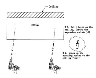
Drill two mounting holes on the ceiling, Install the mounting socket.
