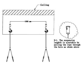
Screw on two suspension ropes to the mounting sockets.
