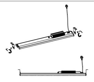
3. Flip the mounting brackets 180 degrees and screw back to the body tightly.
