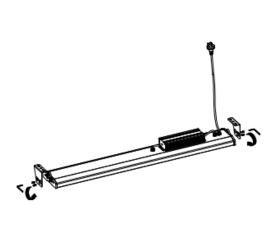
2. Remove the two mounting brackets from the body.
