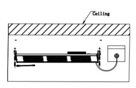
4. Mounting the luminare to the ceiling with expansion screws, plug into the power socket.
