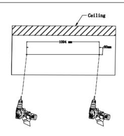
1. Drill 4 mounting holes on the ceiling as per above dimensions.
