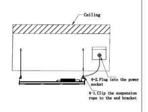
4. Clip on the fixtures and switch on.
