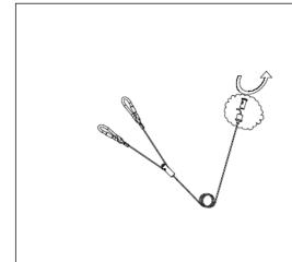
Release the mounting socket of suspension rope as above.
