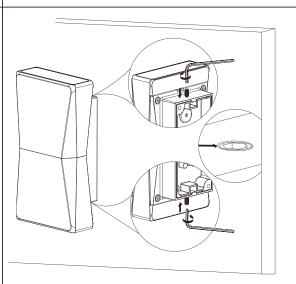
6. Align the body and back cover carefully and lock the top and bottom screws.
