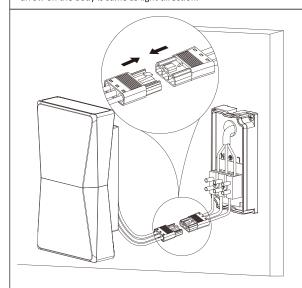
5. Connect the quick connector between back cover and body.
