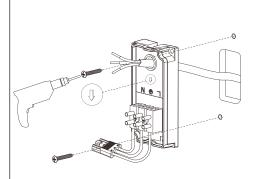
3. Pass the power cable through the grommet and mount the back cover on the wall. ATTENTION: for single head, the direction of the arrow on the body is same as light direction.
