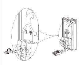
4. Connect L/N/E cable to the terminal block firmly.
