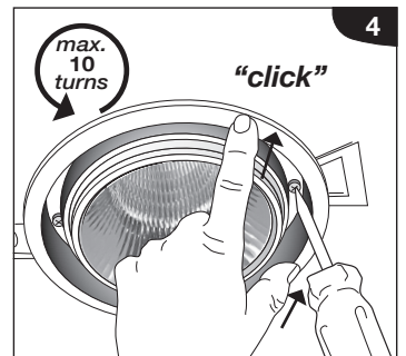
4. Repeat Step 2 by unscrewing second beam direction locking screw.*
