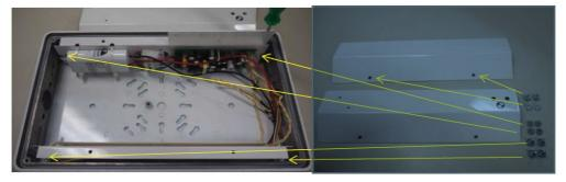
Remove back plate and replace (4) screws with (4) supplied nuts and screws
