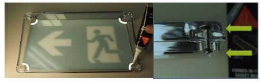
Place pictograph on to diffuser and apply clear silicone to Install to each corner
