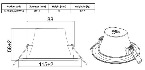
**3. INSTALLATION / GENERAL:** Installation of the product is to be completed by an authorized and licensed electrician, in accordance with these instructions, relevant Australia standards and local regulations (where applicable). Termination of product wiring, together with the installation of the product must be in a manner and orientation that maintains the integrity of the designated IP rating of the product for electronic control equipment (when supplied) DO NOT MEGGER between A and N.
