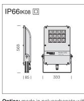
**Optics:** made in polycarbonate with high-efficiency PVD metal surface finishing.
