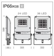
Reflector: in PMMA, highly resistant to temperature and UV radiation.
