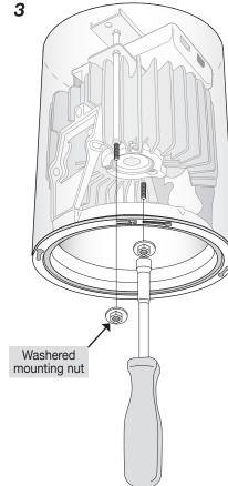
Secure luminaire with washered mounting nuts (tool supplied). Caution - do not over tighten
