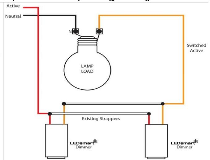
Rocker switches replaced with LEDsmart<sup>+</sup> dimmers using the existing strapper wires. No new wiring required.
