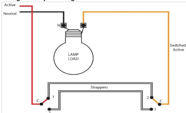
Traditional two-way switching using standard rocker switch mechanisms and strappers between the switches.
