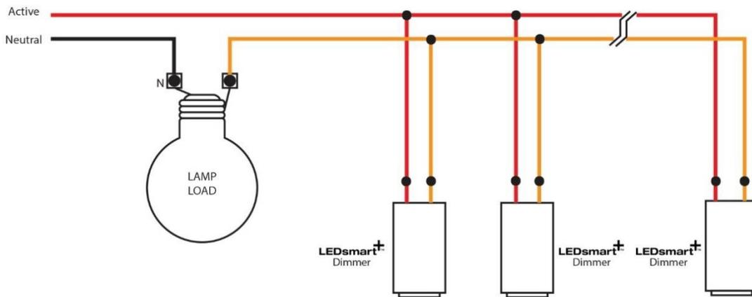
Three-way dimming and switching using LEDsmart<sup>+</sup> dimmers. Note that each two-wire LEDsmart<sup>+</sup> dimmer is simply wired in parallel.
