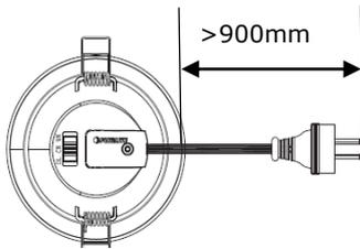
2. Select the colour temperature from the downlight WW 3000K, CW 4000K, DL 6500K using the dip switch on the downlight.
