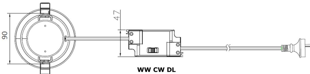
3. Fold spring clips and push into cut-out
