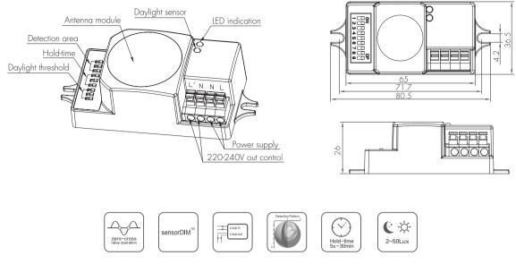
Note: We recommend the mounting distance between sensor to sensor should be more than 2m to prevent sensors from false-triggering.
