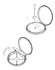
Step 4: Put cable through the entrance hole and connect it to the terminal block. Adjust the CCT as per the requirement 3000k/4000k/5700k
