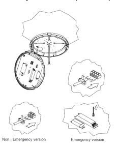
Step 5: Position and fix the base onto the ceiling
