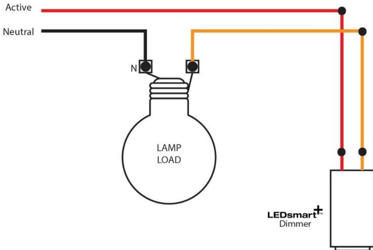
**Replacing existing one-way switch with one-way switching/dimming**
