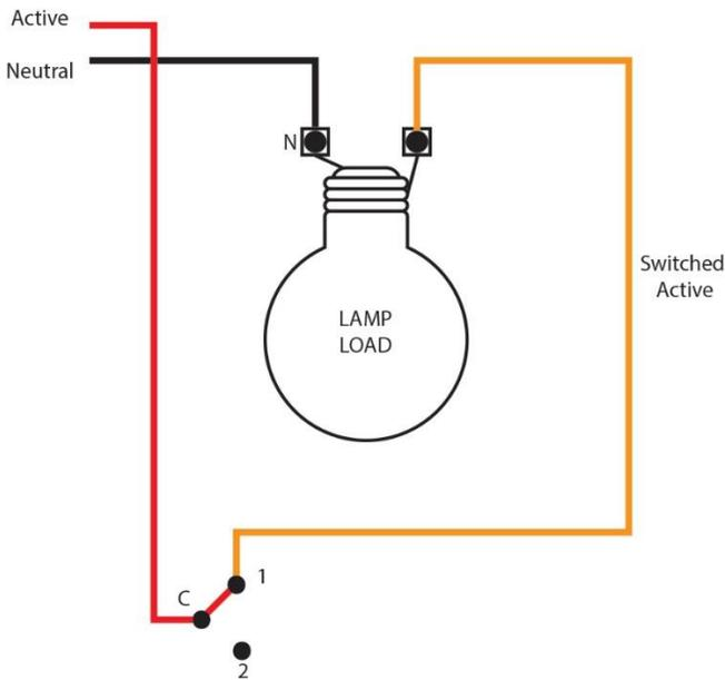
Replacement one way dimming/switching
