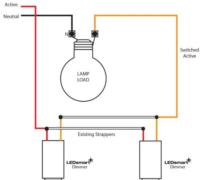
Rocker switches replaced with LEDsmart+ dimmers using the existing strapper wires. No new wiring required.
