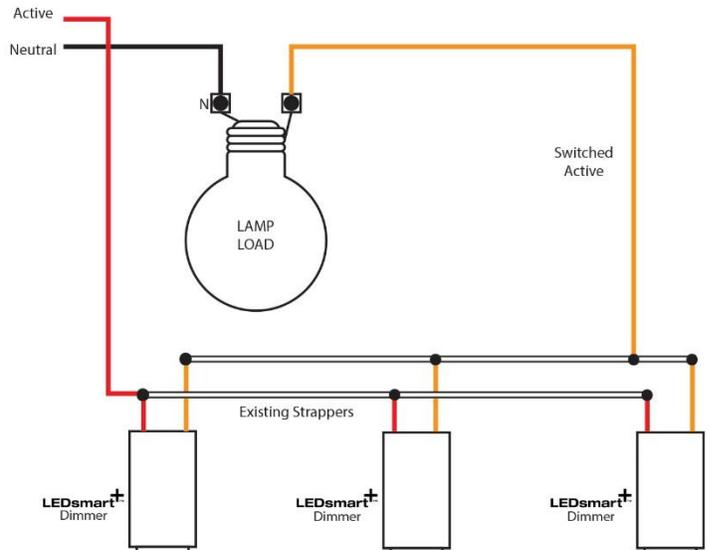
Rocker switches and intermediate switch replaced with LEDsmart<sup>+</sup> dimmers. The existing strappers are used to connect the dimmers in parallel. No new wiring is required.
