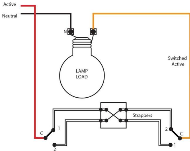
Traditional three-way switching using two rocker switches and one intermediate switch, with strappers between the switches.
