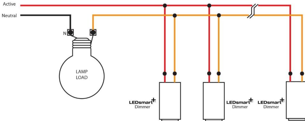
Three-way dimming and switching using LEDsmart<sup>+</sup> dimmers. Note that each two-wire LEDsmart<sup>+</sup> dimmer is simply wired in parallel.
