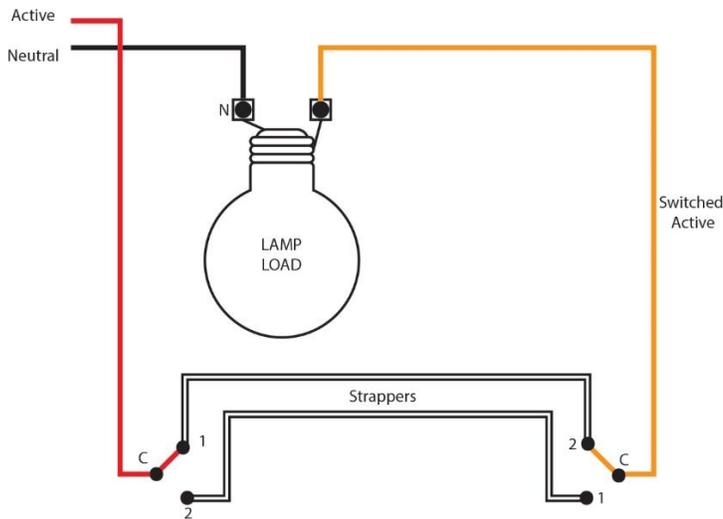
Traditional two-way switching using standard rocker switch mechanisms and strappers between the switches.
