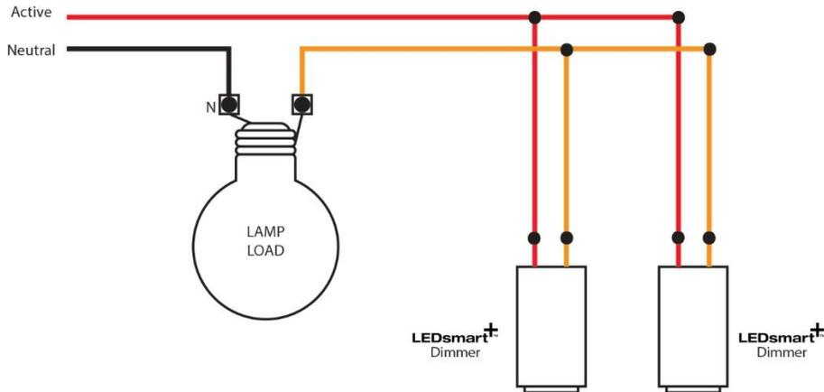
Two-way dimming and switching using LEDsmart<sup>+</sup> dimmers. Note the two-wire dimmers are simply wired in parallel.
