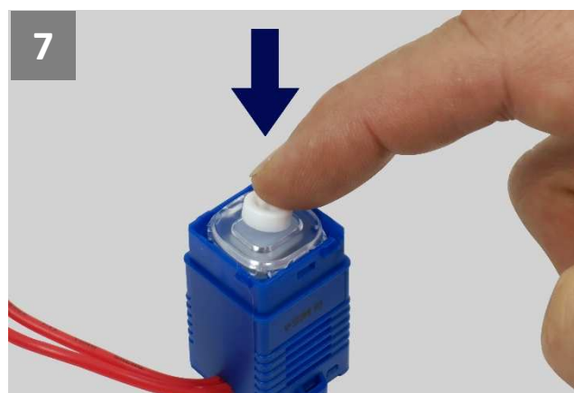
7 Push the pin on the adaptor through the hole on the silicon button
