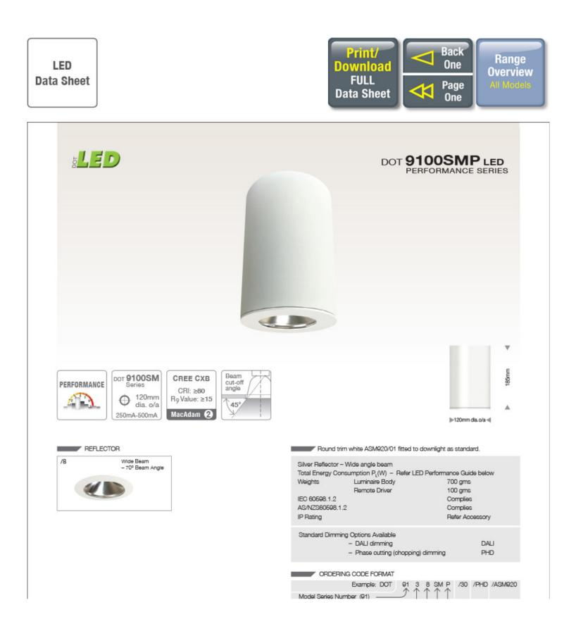
Driver Code (2: 250mA, 3: 350mA) Beam Angle (8-Wide) Downlight Type (SM-Surface Mounted) Series Code (P: Performance) LED engine colour (30-830 or 40-840)
