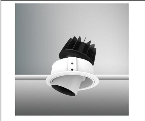
The Dixi Snoot recessed downlight is an architecturally appealing low glare alternative to the standard downlight. It features a 20 degree tilt and 355 degree rotation. The Snoot component reduces glare and minimises light spill as well as being a distinctive attribute to the downlight. Suitable for use in retail, display, commercial, and hospitality.
