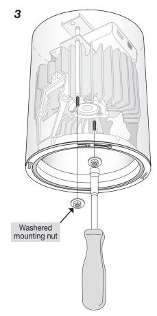
Secure luminaire with washered mounting nuts (tool supplied).
