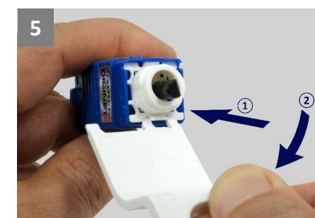
5 Firmly push the tool into the two holes, then rotate the tool away from the housing to release the Rotary Retaining Ring. Repeat the process on the other side of the housing.
